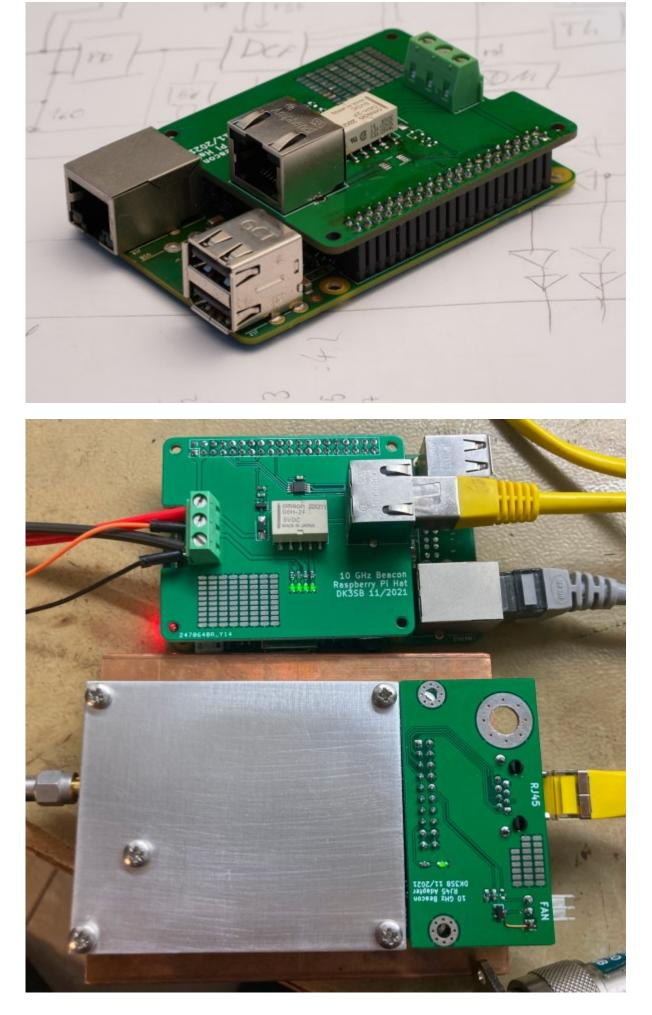
The transmitter and its slot antenna were finally mounted on a large heat sink and placed on a base plate. A 10 GHz circulator was added in-line to avoid damaging the TX in case the return loss of the antenna suddenly degrades due to e.g. temporary water intrusion. An outdoor GNSS antenna was mounted adjacent to the transmitter, to be used for the GNSSDO. The whole assembly is enclosed within a (commercial, surplus) fiberglass radome.
