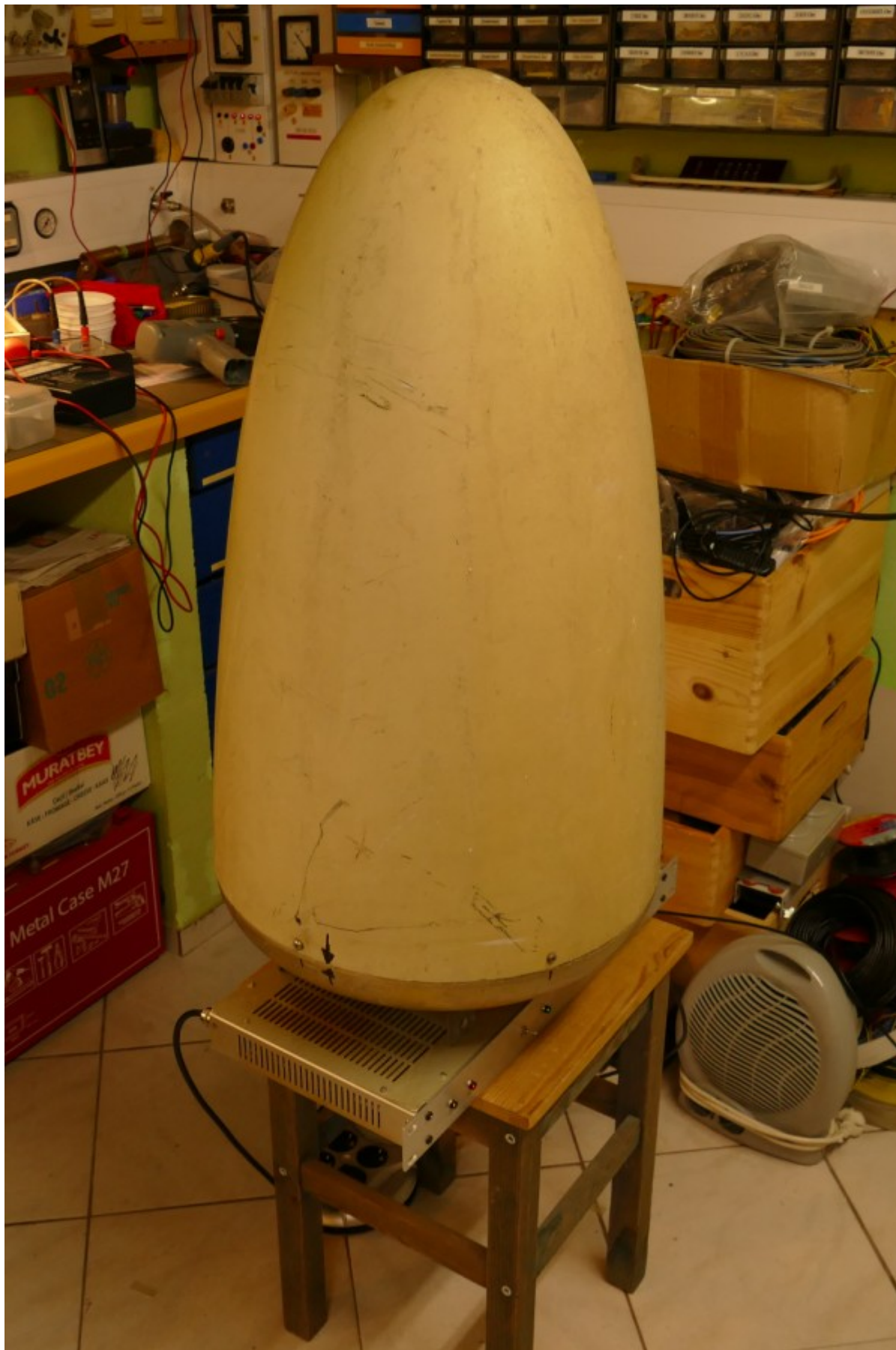
A corresponding indoor unit (19,, rack mount) was manufactured by Rolf DL2ARH. It houses a mains power supply, the Raspberry Pi plus RS-422/supply shield, and a Leo Bodnar GPSDO. The GPSDO is also monitored through its USB interface by the Raspberry Pi for loss of GNSS lock etc.
