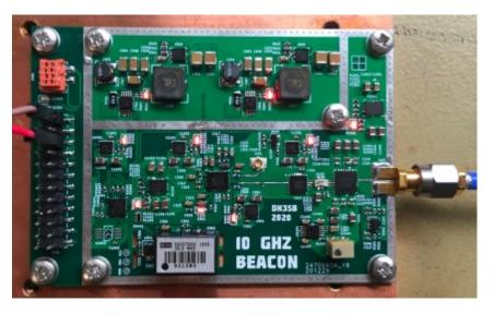
One of the key design features that helps with driving down cost is working with a commercial fourlayer FR4 stackup. These have become ubiquitous and cheap to use, so one supplier (JLCPCB from China) was chosen and their PCB process characterized for RF performance. Two dedicated RF test coupons were designed: Based on the results of long simulations, prototype designs for SMA connector footprints, microstrip, coplanar waveguides etc were designed.
