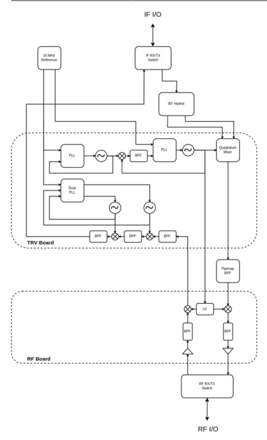
As transceiver IF 50 MHz is used. The transmit path is designed for <1W input power. With a 90° hybrid coupler the quadrature mixer in the transmit section of the transceiver module is used as a image reject mixer to 2.63 GHz. This IF gets filtered externally with a 28mm pipe cap filter to further attenuate the LO and side-band signal (+harmonics). In the first built 0.5 W output power could be reached without additional tuning of the power amplifier. The receiving chain consists of 3
