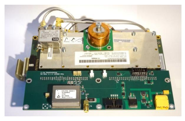
First all the details of the modules were reverse engineered(documented here in german) and a concept for the usage as a 3cm transverter was worked out. A first prototype was tinkered together and performed very well:
