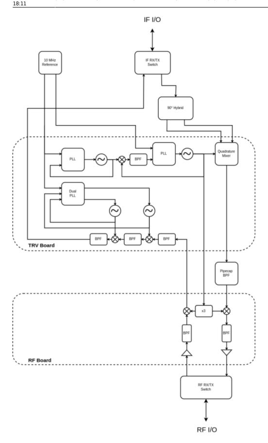
As transceiver IF 50 MHz is used. The transmit path is designed for <1W input power. With a  $90^{\circ}$  hybrid coupler the quadrature mixer in the transmit section of the transceiver module is used as a image reject mixer to 2.63 GHz. This IF gets filtered externally with a 28mm pipe cap filter to further attenuate the LO and side-band signal (+harmonics). In the first built 0.5 W output power could be
