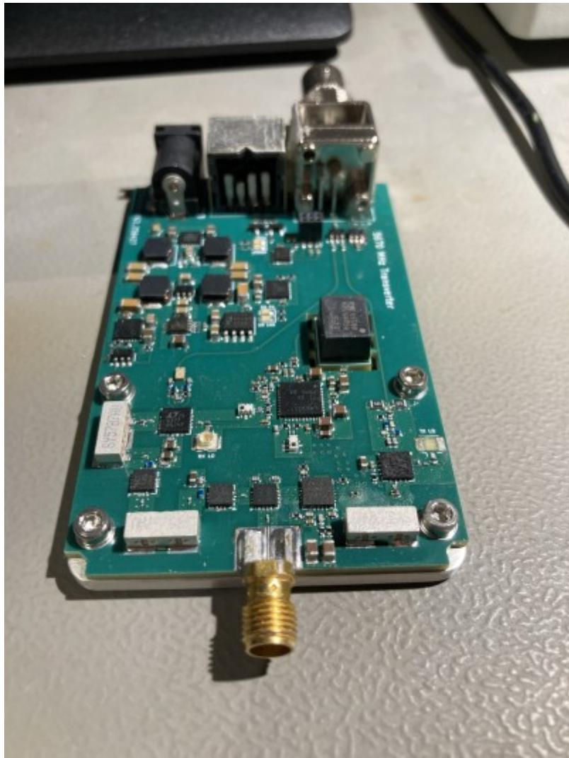
In transmit mode 7.5 watts of heat is dissipated. For proper heat sink the PCB is directly connected to the housing with attached heatsink.
