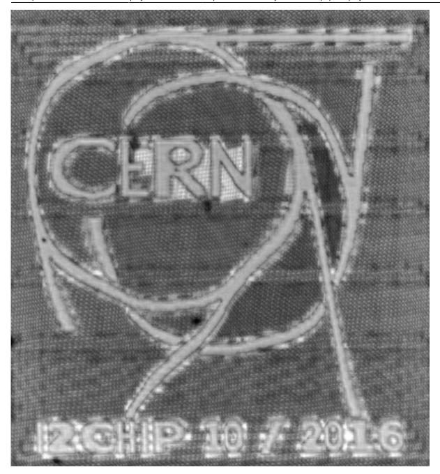
This picture shows some of the aforementioned nonlinearity in one axis, which introduces periodical distortions in the image. These could be corrected in principle, but I didn't bother. The nice CERN logo was placed on the top metal layer, and is composed of many small pixels that are on the order of a few micrometers large.
