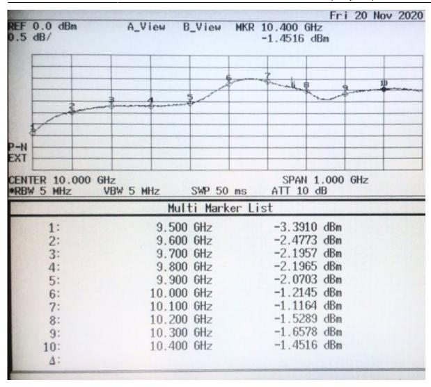
Spectral content was verified at 10.368 GHz to be in line with the datasheet typical values:
