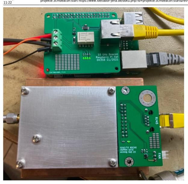
The transmitter and its slot antenna were finally mounted on a large heat sink and placed on a base plate. A 10 GHz circulator was added in-line to avoid damaging the TX in case the return loss of the antenna suddenly degrades due to e.g. temporary water intrusion. An outdoor GNSS antenna was mounted adjacent to the transmitter, to be used for the GNSSDO. The whole assembly is enclosed within a (commercial, surplus) fiberglass radome.
