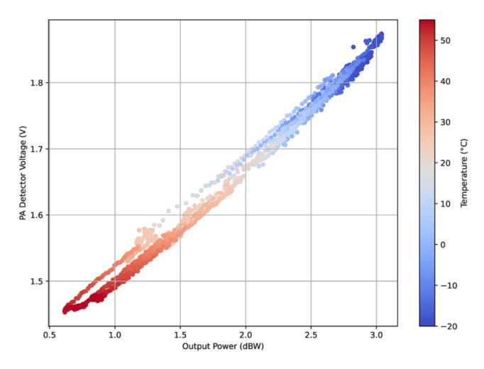
Across the full temperature range, the output power was found to vary by about 2.5 dB. This is not untypical for a fixed gate voltage design without temperature compensation. The negative temperature coefficient ensures there is no thermal runaway at high temperatures, and with a peak RF output power of 2 W at -20°C, there is enough operational margin for some reduction at higher temperatures, aging, etc.
